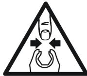
Use of an open end front part with this tool can cause crushing of fingers and hands.
