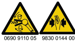
Check the rotational direction of the tool before start! A start in an unexpected rotational direction can cause bodily injury or property damage. Moving parts can crush and cut.
