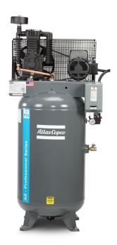
AR piston Compressors are splash lubricated, two-stage compressors with a maximum operating pressure of 175 psi. All models feature an aluminum pump. Models are equipped with a magnetic starter, low oil level switch, and pneumatic auto drain.
