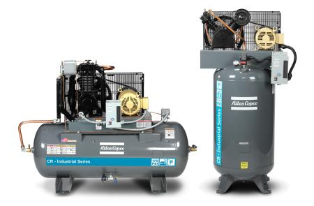
CR piston compressors include a cast-iron pump and are splash lubricated, two-stage compressors with a maximum operating pressure of 175 psi. All models feature a magnetic, electronic auto drain, low oil level switch, and belt guard-mounted aftercooler.
