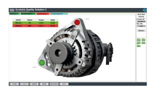
The SQS3 Operator Guidance drives the assembly workflow at the workstation.
