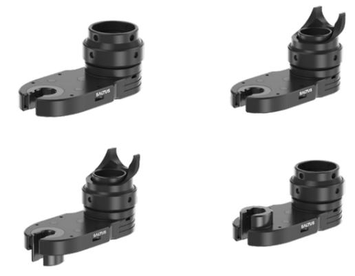
Models are available in a number of gear stages which allow for length extension, helping to reach difficult-to-access joints. Narrow models offer the possibility of reaching several tube nuts concentrated in small areas such as on ABS control module installations in vehicles.
