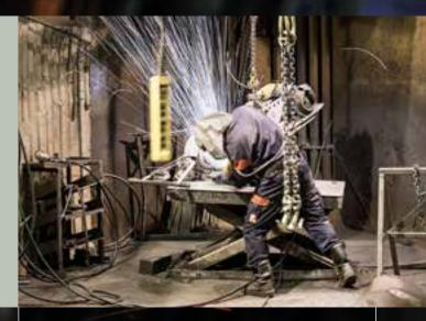
**EFFECTIVE GRINDING** with the right tool makes additional processes unnecessary. Cutting close to the work piece leaving close to nothing behind.
