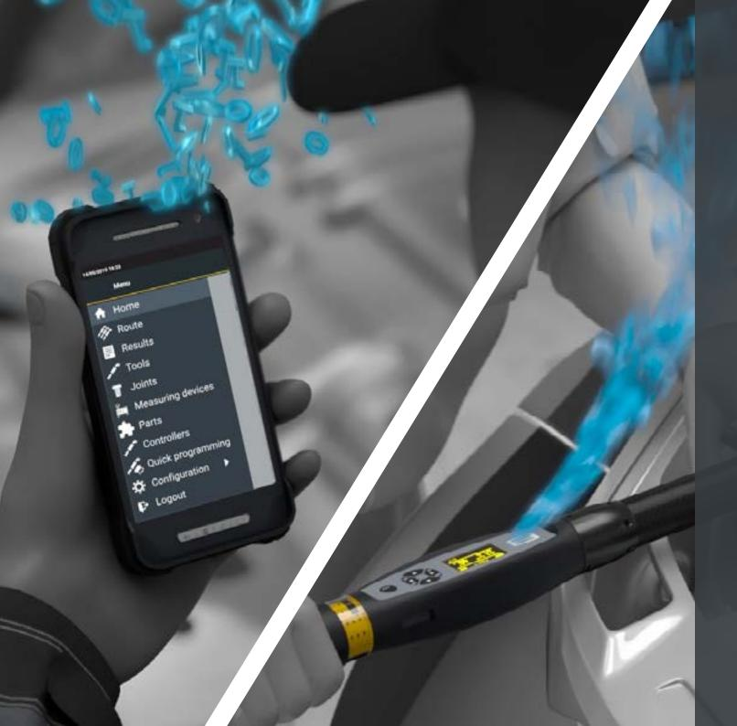
The Joint check programs automatically reach the operator through STpad following the optimized route defined by QA Supervisor.
