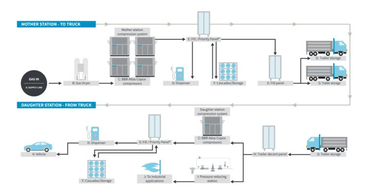
A: Supply line B: Gas dryer C: BBR compressor D: Dispenser E: Fill/priority panel F: Cascades G: Trailer storage H: Trailer decant panel I: Pressure reduction station (PRS) J: To industrial applications K: Vehicle
