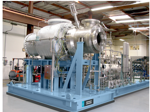
A turboexpander for cryogenic hydrocarbon separation.
