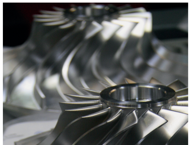
Aerodynamic performance is determined by shape of the blades and tip speed.
