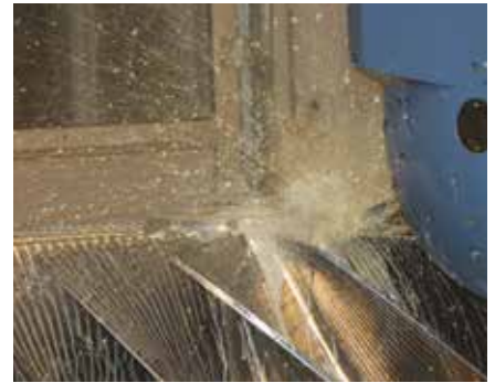
Inside the multi-skill machine: the milling process
