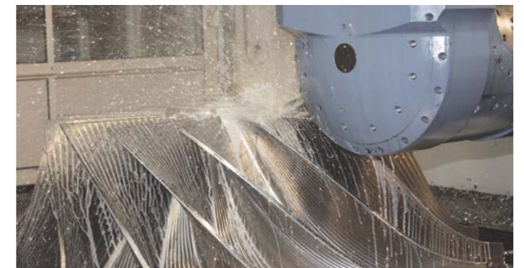
Inside the 5-axis machine: the milling process
